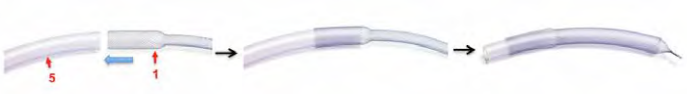
Fig. 5: Pushing of the nitinol braid over the cleaning tube
